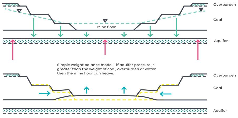
The mine floor yields, water from the aquifer can flood the mine and the batters can also collapse
