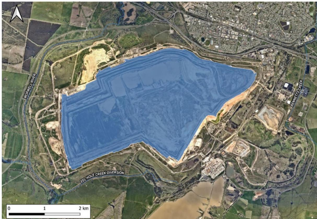
Figure 1 Illustration depicting a lake at +45m AHD at the present-day Hazelwood mine site south of Morwell, as proposed by Engie. All mine infrastructure will be removed and the lake margins rehabilitated to integrate with the surrounding terrain
